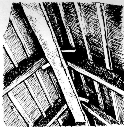
Fig. 55 (a) Danish loose-hung rafters on a building from Fünen at the Frilandsmuseet Open Air Museum Illustration after material in the 1962 Guide to the Museum (b) Ridge of a Fünen house seen from below. The peg ends at the ridge are clearly visible Drawing after a photograph in the Frilandsmuseet Guide
